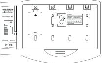
2. Press ANALYZE. The charger displays the estimated charge level, with amount-ofthe charge symbol and the numeric characters showing the voltage.
